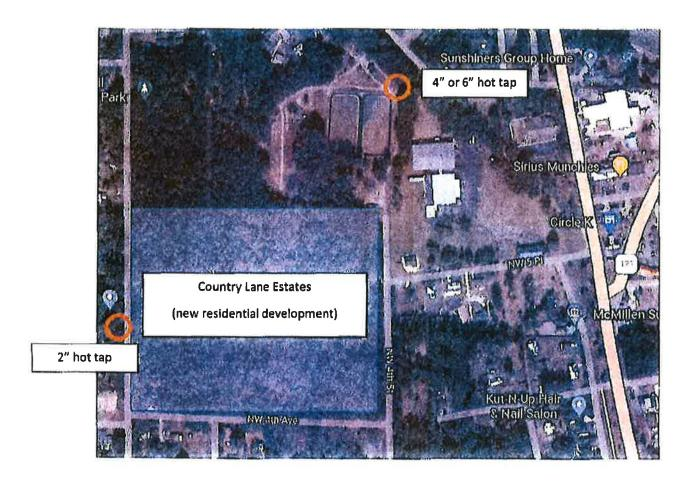
City will need a hot tap on the line coming out of their reg station at the water treatment facility. The line is either a 4" or 6" steel.
