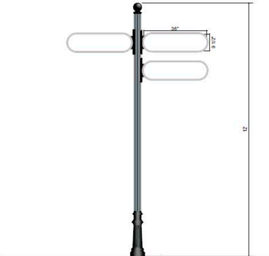
3" fluted post, B-3 finial, SB-33 post and oval 12"x 36" frames, painted black with two 9 1/2" x 36" sign blanks for customer to apply graphic prints.
